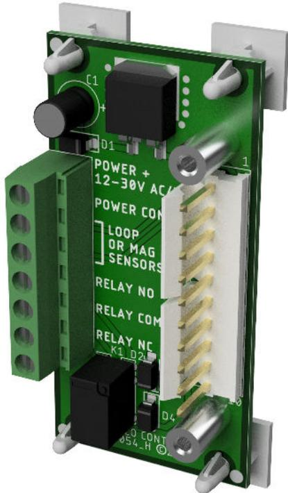
Many vehicle detectors are designed to be plugged into a rack including some of the more popular Diablo Controls models. In those installations where a large rack is not available, Diablo Controls has designed a mini rack. The RK-1R is designed to accept a plug-in vehicle detector on one side and accept the appropriate wires through the terminal block on the other. The entire mini rack is supported by four adhesive standoffs that attach anywhere in the cabinet.
